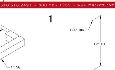
Determine the position and location of the DH3 at the work surface. Drill a 1/4" diameter hole with the recommended on center dimension.
