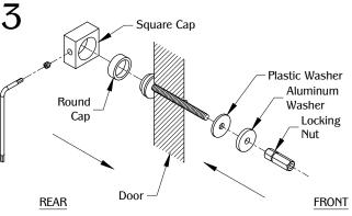
Assemble (1) plastic washer, (1) aluminum washer and (1) locking nut at the front of the work surface. Tighten the assembly. Finish the hardware assembly by installing the round and square cap. Repeat Step 3 & 4 for the other side.
