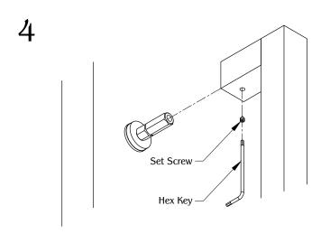
Align the DH3 to the assembled base. Secure it with the (2) set screw using the hex key.
