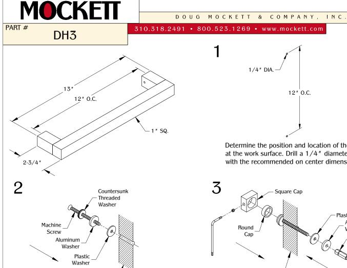
Assemble (1) machine screw, (1) countersunk threaded washer. (1) aluminum washer and (1)plastic washer at the back of the work surface. Align the assembly through the predrilled hole. (Note: Use 4" screw for thicker door.)
