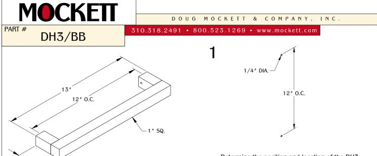
Determine the position and location of the DH3 at the work surface. Drill a 1/4" diameter hole with the recommended on center dimension.
