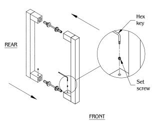
Align the DH3 to the assembled base. Secure it with the (4) set screw using the hex key.
