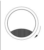
Install the BRV2 lid by aligning the tabs to locking groove and rotating BRV2 lid clockwise to lock.
