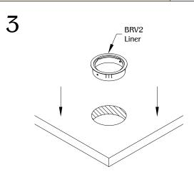
Install the BRV2 liner into the cut out and make sure it is fully leveled on the work surface.
