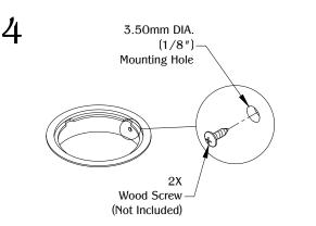
Use (2) wood screws to secure part onto the work surface.(Note: Use appropriate wood screw type and length depending on the material and thickness of the work surface.)
